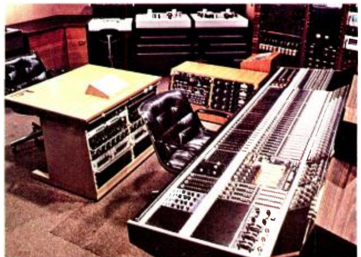
Figure 6. This view of the mix-down room shows the auxiliary equipment rack behind the mixer, mounted in the producer's table.
